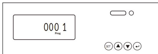
**Step 3:** Click the "Enter" button to enter the above interface, and press the up and down arrow keys to enter the password 0001.
