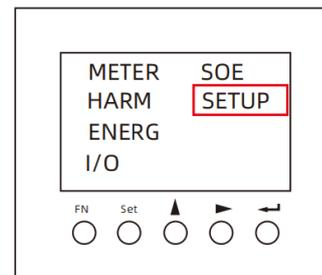
**Step 1:** Activate the meter display by pressing any key. Then click the "Set" button.
