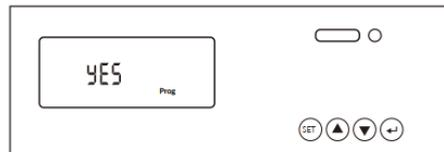
**Step 10:** Click the "Enter" button to enter the following interface, press the up and down arrow keys, and set "no" to "YES" to save the configuration.
