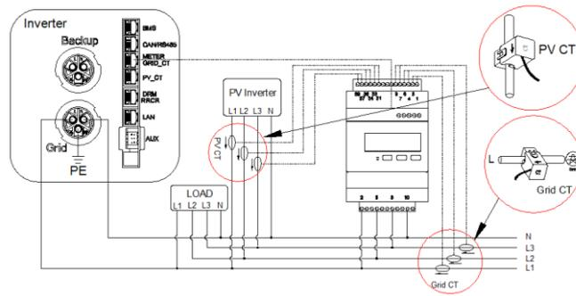
Wiring at three-phase feed in
