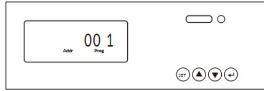
**Step 6:** Click the "Enter" button and press the up and down arrow keys to set the meter address. The Grid meter (DC, AC and Hybrid system) address is set to 001, the PV meter (AC and Hybrid system) address is set to 002.
