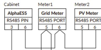
**!** **NOTE:** If the ADL3000 meter with CT is used as a grid meter, the direction of arrow in CT should point away from the grid to the energy storage system. If the ADL3000 meter with CT is used as a PV meter in AC- or hybrid-coupled system, the direction of arrow in CT should point away from the PV inverter to the energy storage system.
