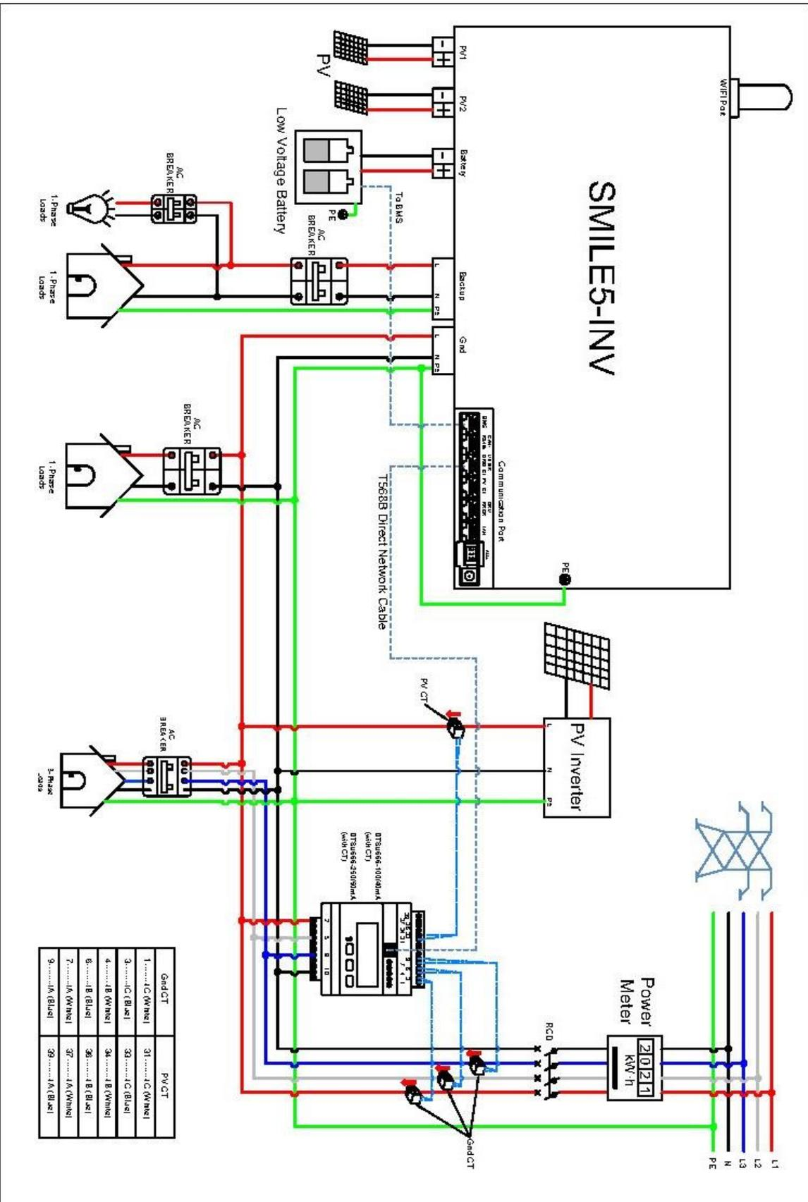
3.SMILE5 System Wiring Diagram with CHINT Electricity Meter DTSU666 (Without CT)
