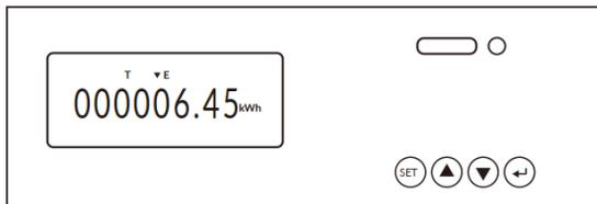
**Step 1:** The initial interface of the meter (normal working mode) is shown above.
