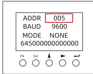
**Step 5:** Set the communication address and communication baud rate in the communication setting interface. When the meter is used as Grid meter (DC, AC/Hybrid system), the address is set to “005” . When it is used as the PV meter (AC/Hybrid system), the address is set to “006” . The baud rate is set to 9600.
