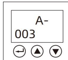
**Step 4:** Please set the meter address by using the “Value adjustment” button, the Grid meter (DC, AC and Hybrid system) address is set to 003, and the PV meter (AC and Hybrid system) address is set to 004.
